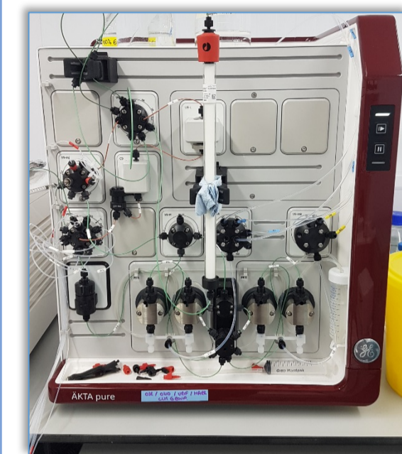
Fig.2) AKTA pure™ chromatography machine, used for affinity purification of MBI5 from cell supernatant
